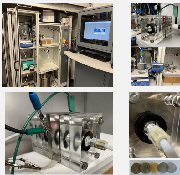
Figure 16: Flow-Through Setup for electrochemical characterization created in TU Claustahl
